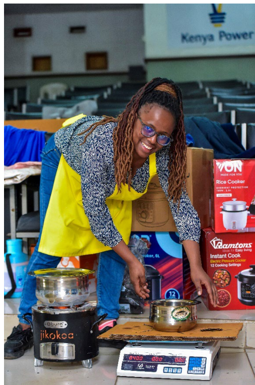
Figure 1: Collecting data on fuel consumption during the Controlled Cooking Tests (CCTs).
