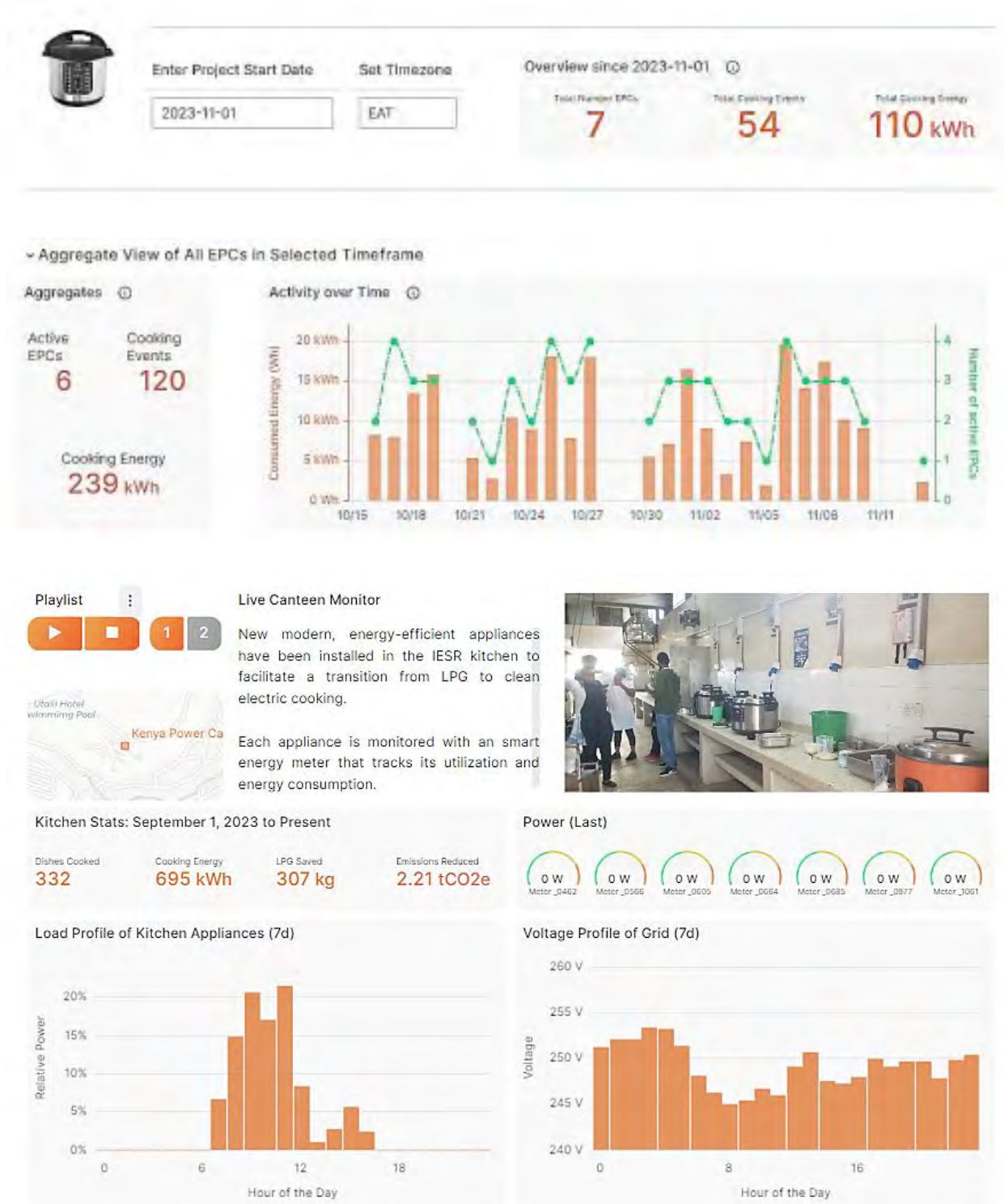
Figure 21: Appliance Demand Platform (ADP) dashboard for the appliances installed in the IESR kitchen showing metrics for individual EPCs and the energy used to prepare the meals being served.
